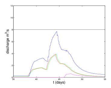
Figure 3.11: Discharge rates with weir height 0.6 m and initial ditch level 0.25 m for one subcatchment (red).
