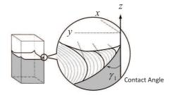
Figure 4: Contact angle at corner (courtesy of Weislogel and Lichter JFM 1998).
