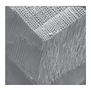
Figure 3: Image of tracheids of conifers.
