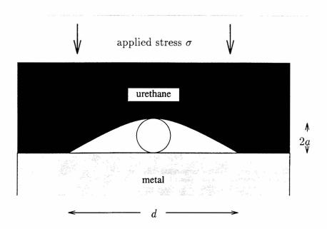
Figure 6: Schematic diagram of a trapped proppant particle
