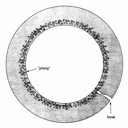
Figure 4: Schematic diagram of the wear pattern in a failed seal
