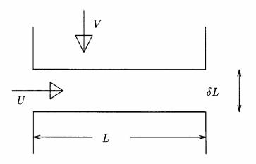
Figure 5: Definition sketch for the inviscid squeeze film
