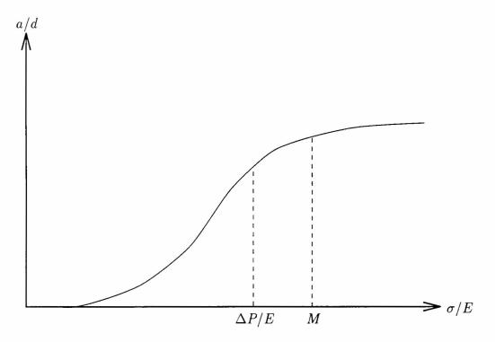
Figure 10: The relationship between applied stress and contact distance
