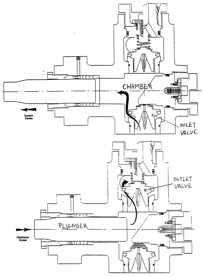
Figure 1: A two-stroke positive displacement pump
