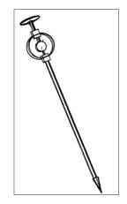
Figure 18. A modern penetrometer [3]
