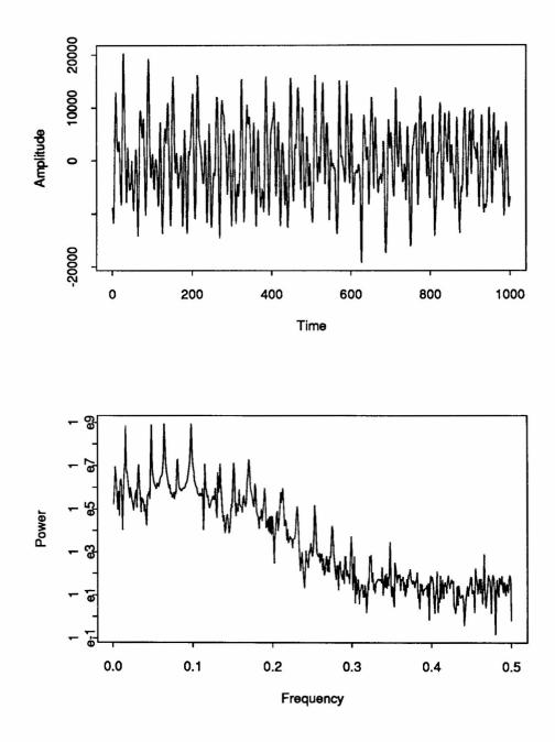
Figure 1: (a) Plot of 1000 observations (0.02 secs) of piano music. (b) The periodogram (squared amplitude of Fourier coefficients of the data plotted in (a)).
