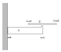
Figure 10. A sketch of load cell (1) plus steel plate (2). The fruit carrier slides along the top plate, from the rear to the front, at roughly constant speed, while it is being weighed.
