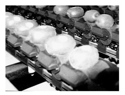
Figure 1. Kiwifruit in their containers. Movement is right to left. Each container can rotate fruit, tip fruit out, and float free of the chain (vertically) while being weighed.
