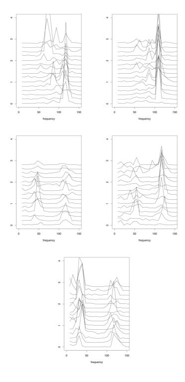
Figure 7. Frequency spectra for 5 different standard fruit weights (137.2g, 200g, 293g, 403.5g and 573g) at a line speed of 300cpm.
