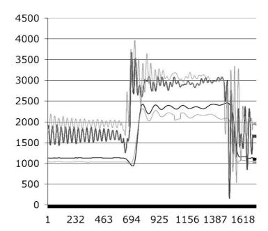
Figure 5. Voltages from the two load cells, as a 513g imitation orange and its container cross at 5 fruit/second (0.5 m/s). The two larger signals are the raw data, and the two lower amplitude signals are the outputs from the analogue low-pass filters used by Compac.
