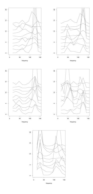
Figure 8. Frequency spectra for 5 different standard fruit weights (137.2g, 200g, 293g, 403.5g and 573g) at a line speed of 600cpm.
