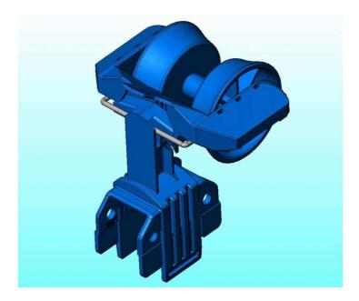
Figure 2. Detailed drawing of a fruit carrier. Towing direction is right to left. The top part floats independently of the lower part, when on the loadcell.
