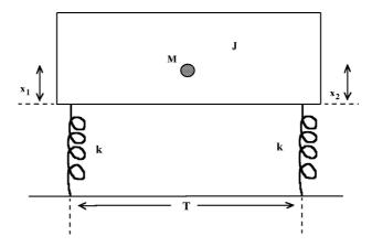
Figure 6. A sketch of our simple model, incorporating up-and-down motion plus rocking from side to side.
