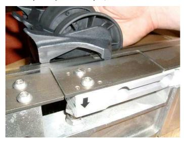
Figure 3. A loadcell with the steel plate on top, and a (handheld) carrier moving over it from right to left. Note the two tracks worn into the steel plates by the moving contact points of the carrier.
