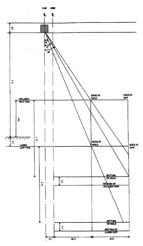
Fig. 1. Geometry associated with the largest ships (dimensions in m).
