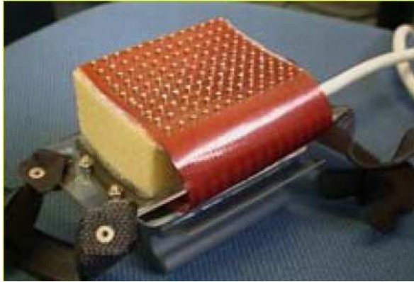
Figure 4: High-density sEMG setup. This setup records up to 130 channels at once.
