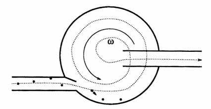
Figure 1: Sketch of the cyclone separator.
