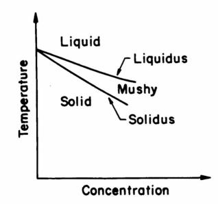
Figure 2: Typical solidification behaviour in the presence of impurities
