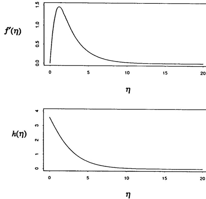
Figure 2: (a) Non-dimensional velocity  $f'(\eta)$ . (b) Non-dimensional temperature  $h(\eta)$ .
