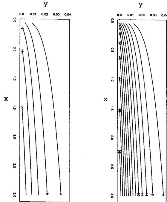
Figure 3: Temperature contours below the interior ambient temperature  $T_\infty$  (a)  $q_w = 50 \text{ kW/m}^2$  (b)  $q_w = 150 \text{ kW/m}^2$ .
