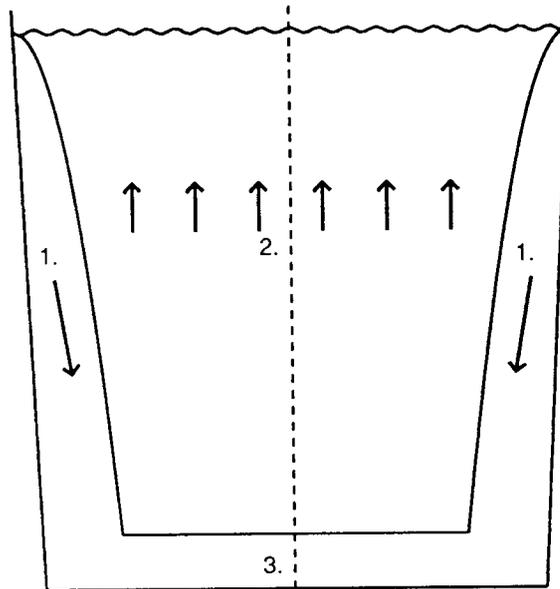
Figure 1: Zones of flow predicted to form in a ladle under natural convection: 1 is the wall boundary layer zone, 2 is the central or core zone, and 3 is the quiescent zone.
