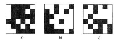
Figure 12: Matching of code matrices. Matching cells marked. a) Fig 11a vs. Fig 11b (same fingerprint): 66% match; b) Fig 11a vs. Fig 11c (different fingerprints): 44% match; c) Fig 11b vs. Fig 11c (different fingerprints); 42% match.
