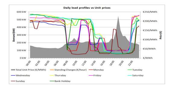
Figure 16: Load profile of a customer with a cold storage facility
